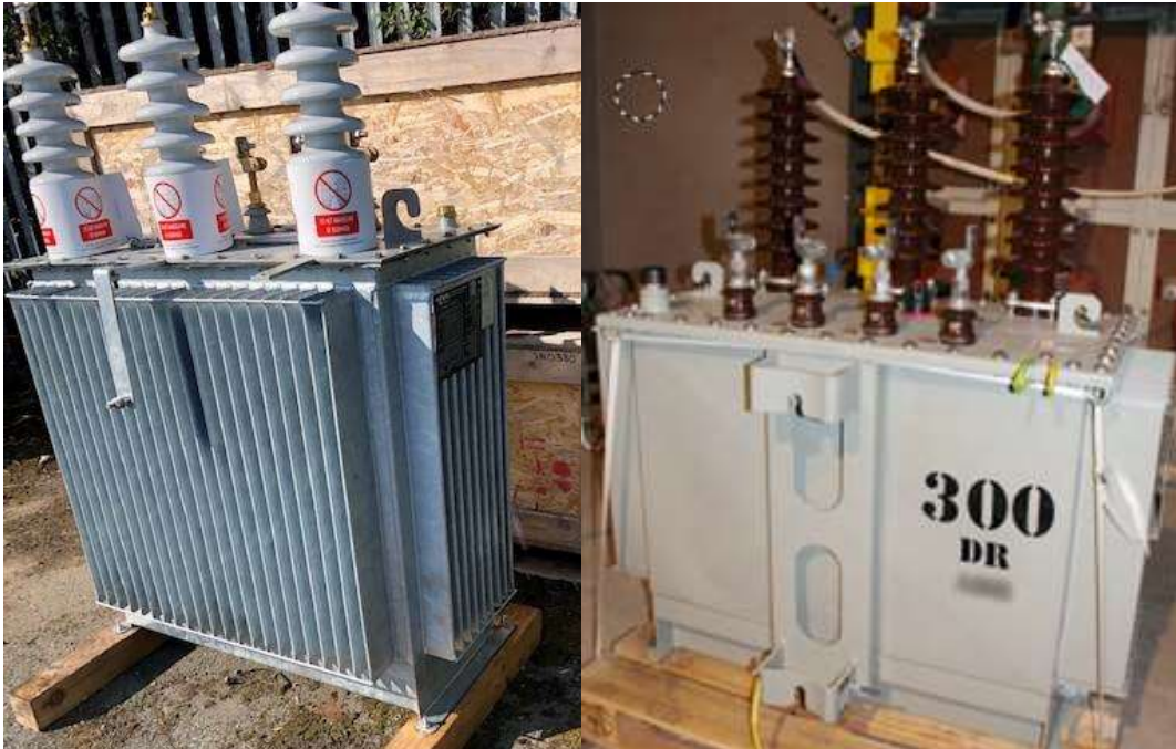
Figure 1: Photographs of the 300 kVA pole mounted transformers from the two suppliers
