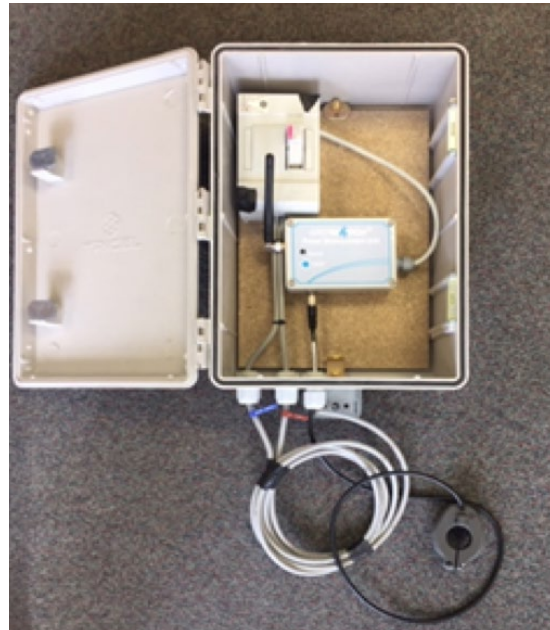
FIGURE 8 INSIDE POLE MOUNTED MONITORING DEVICE DEVELOPED BY MAC DEVICES
