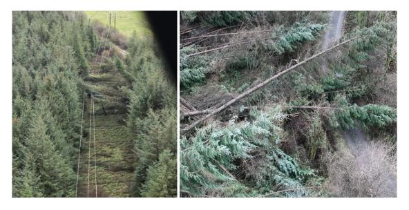
The extent of customer faults and network damage resulting from falling timber in our recent storms has also been overlaid to identify the network most vulnerable to falling trees. In total, of the 3,112km of medium voltage network running through forestry, 710km are most at risk for this winter (see table below and associated note). While this risk is most acute on the medium voltage network some residual risk also remains on the 38kV network.
